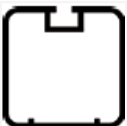
Poteaux section 80 x 80 mm
